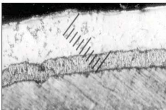
Microstructure of zinc hot-dip galvanized wire
